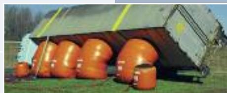
When emergency equipment is required, TNT will dispatch a special trailer with everything needed for recovery. Shown above: air cushions uprighting a trailer safely and without further damage. TNT's skid-steer loader and portable ramp handle off-loading, transfers of loads, and time-sensitive emergencies such as refrigerated cargo.
